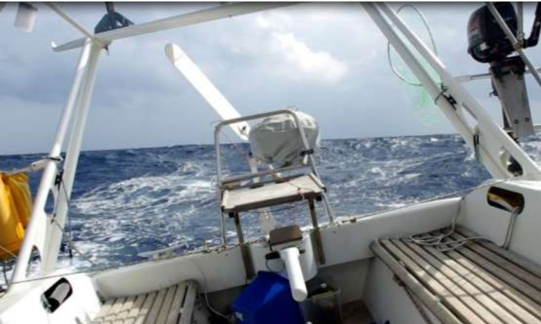
On ocean passages over 90% of time the wind vane steers, close to shore always the electrical autopilot.
